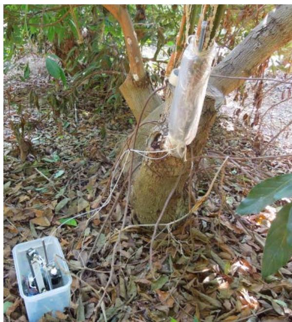
Fig. 6. Collection of volatiles from inside plastic oven bag with air drawn through charcoal filter (top right) and absorbed by Porapak Q filter using 12V vacuum pump.
